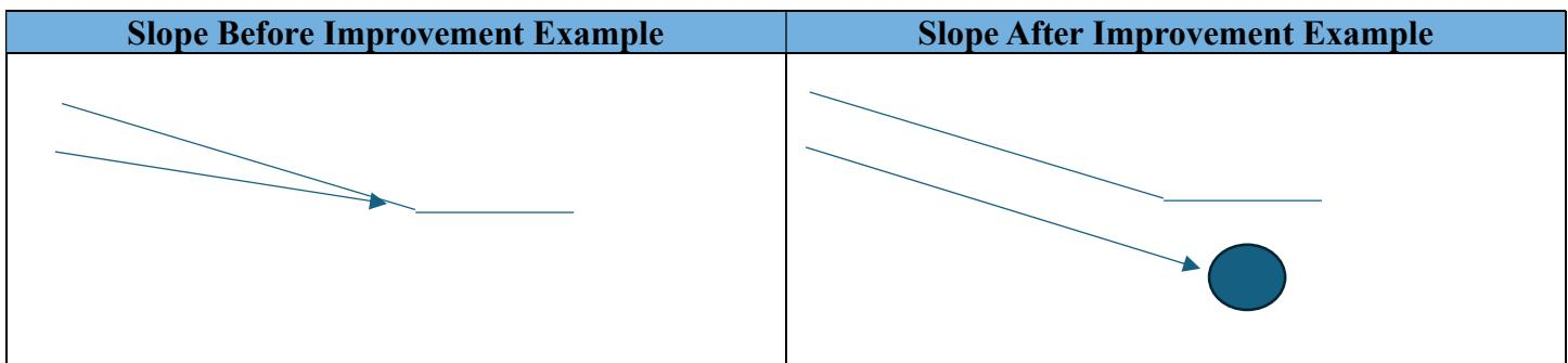
As illustrated above; by installing a tile, a drainage district effectively increases the available "fall" or slope for a private tile system. This allows a landowner to drain otherwise flat or depressional areas and enables them to use smaller, less expensive tile to achieve the same drainage capacity, a direct economic benefit.
