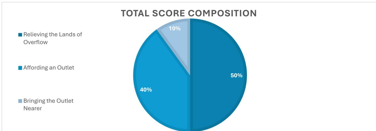
These weights were chosen to emphasize the core purpose of the drainage system, removing excess water from poorly drained soils, while also acknowledging infrastructure use and proximity benefits.
